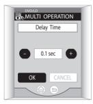
• If you want to change the delay time after it's been set, press the delay time, then press **SET** to come back to this screen.
